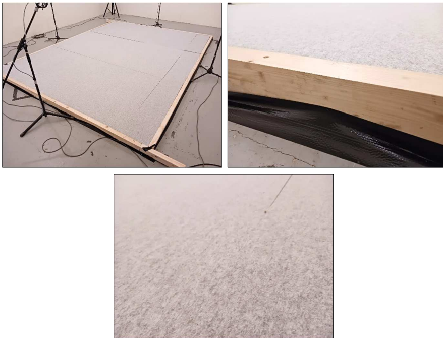
Images 3 to 5 Test specimen installation into the reverberation room
